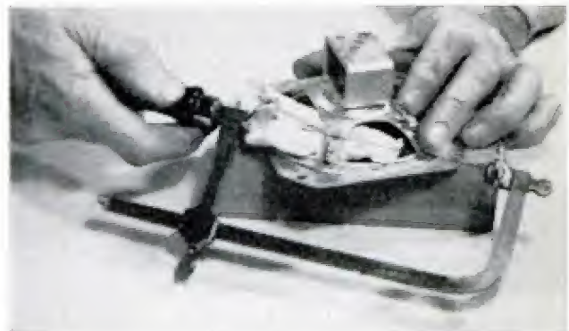
COARSER BLADES can be used for cutting wood, but because of set, they often do not clear themselves
